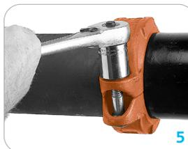
**CAUTION:** Uneven tightening may cause the gasket to pinch. Gasket should not be visible between segments after bolts are tightened.
